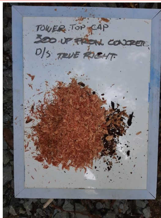
Figure 4. Downstream tower cap drilled in 250mm from tower support through soffit
