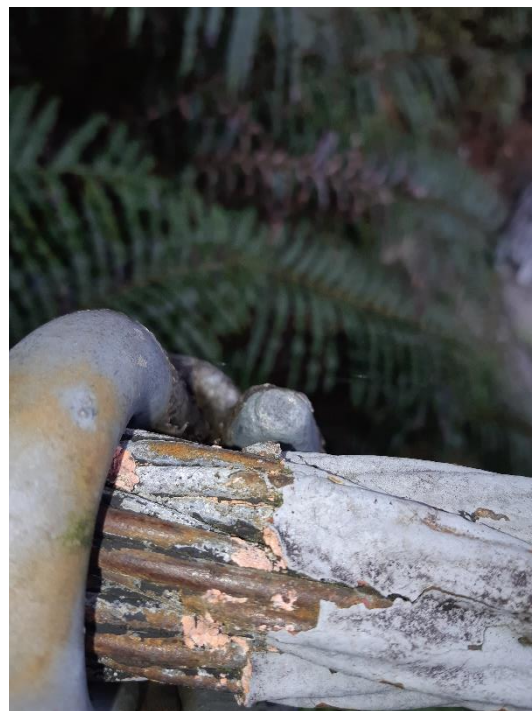
Figure 12. Typical coating damage adjacent to new clamps (not slippage)
