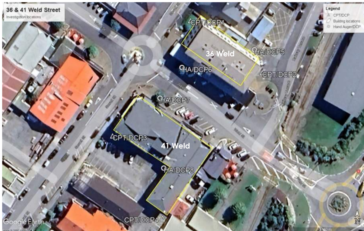
Figure 2. Geotechnical investigation locations for 36 and 41 Weld Street.
