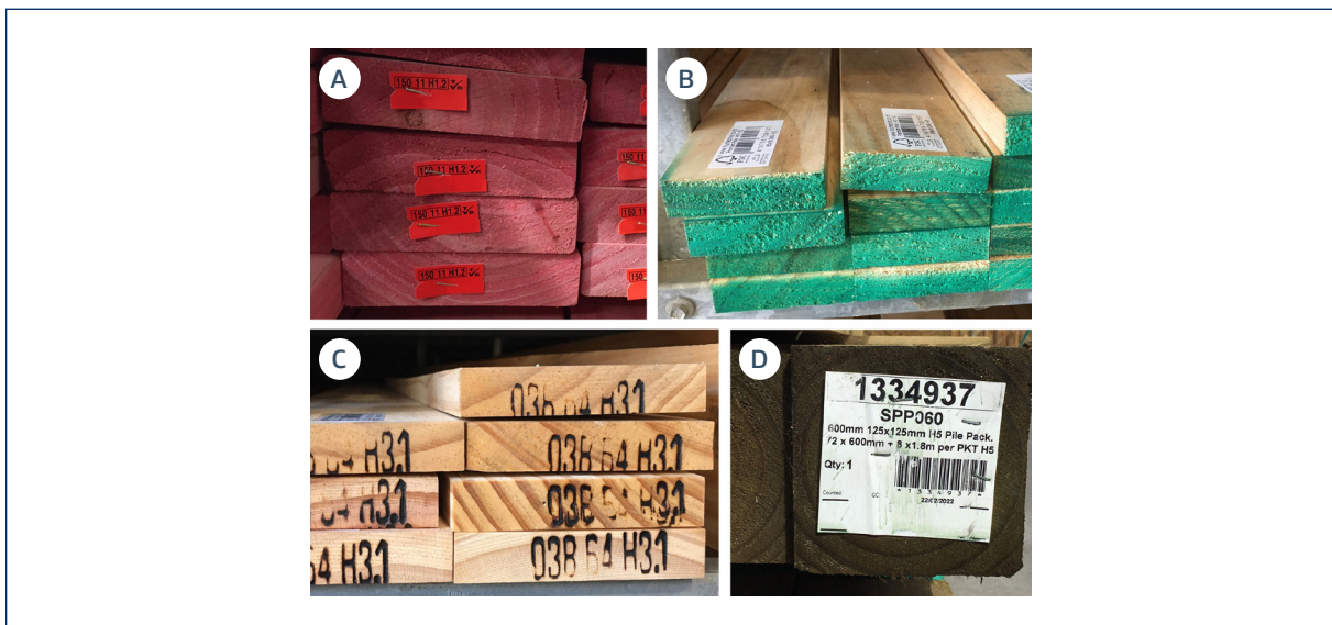
Figure 21. Timber treatment identification. (A) H1.2 timber colour and tag. (B) H3.1 timber colour and marking. (C) H3.1 treatment marked on end. (D) Tag indicating H.5 treatment
