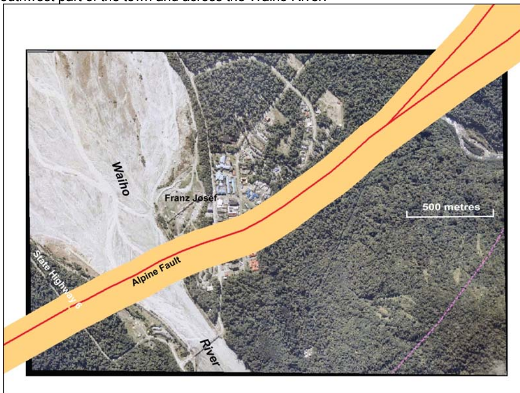
Figure 20 The Fault Avoidance Zone (FAZ) for the Alpine Fault in the Franz Josef area (scale extracted from GIS at 1:9000). Both the new mapped fault trace and the dashed WCRC line occur within the FAZ. In terms of future planning and consenting, a zone of width of 190m is currently placed through the town until better mapping data becomes available.
